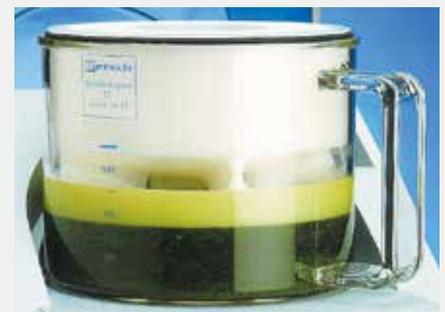
The gravity lid reduces the volume of the grinding container, thus allowing for thorough homogenization of the complete sample.
