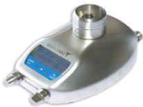
= Enhanced safety burner with IR sensor
