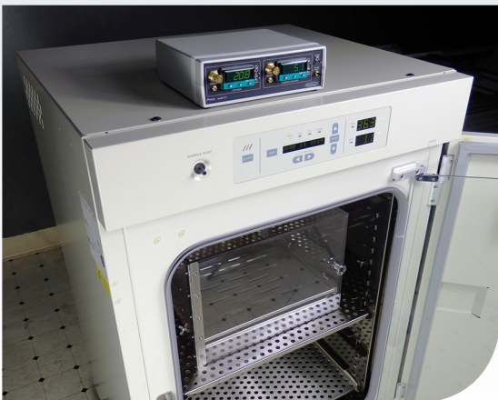
ProOx C21 consists of two basic parts connected by an umbilicus: the controller itself and its adapter pod that attaches to a C-Chamber.
