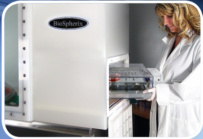
Buffer chamber has two main functions. It acts as an airlock, isolating inside from outside ...
