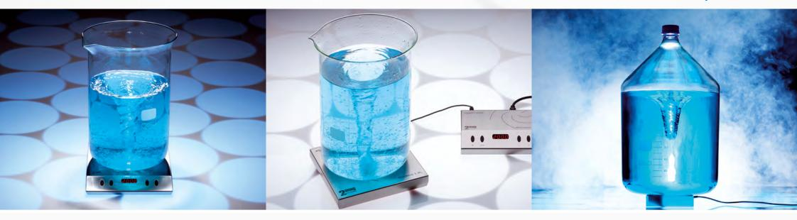
An absolutely innovation is the integrated contact-free stirring bar control mixWATCH. In case of the magnetic coupling is separated between the magnetic stirrer and the stirring bar during the acceleration phase e.g. caused by to high set speed or changing viscosities, the magnetic stirrer will be stopped, the stirring bar centred and started again.
