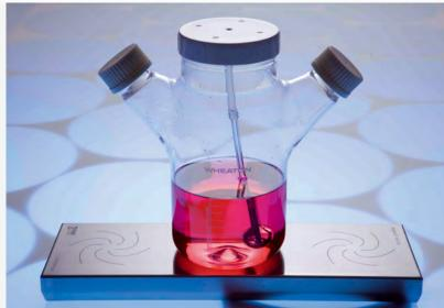
INDUCTIVE DRIVE -MAINTENANCE- AND WEAR-FREE Our magnetic drives are working on the inductive principle. This means that instead of conventionally problematic motors with pull magnets, 2mag is working with stationary coils, which are defined flown through by alternating currents. The thereby generated electromagnetic rotating field is 100% wear- and maintenance-free.
