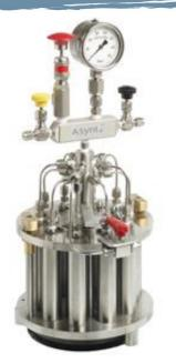
A cost effective, lightweight unit suitable for numerous stirred or non stirred applications. These include hydrogenations and applications where air sensitive materials are used or any other reaction where pressure or temperature are required.
