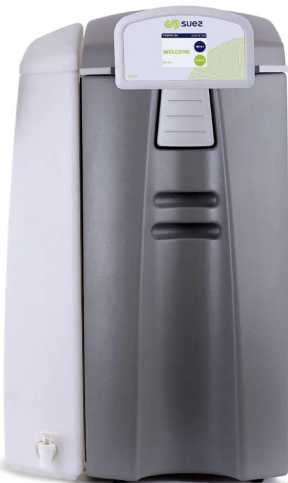
The Purite edi 60 is a compact unit ideal for laboratory use delivering a constant supply of  $>5\text{M}\Omega\cdot\text{cm}$  pure water for laboratory tasks using activated carbon pre-treatment, double pass reverse osmosis, carbon dioxide membrane degassing and electro-deionisation technology. Typical applications include, glassware rinsing, buffers, and stains, reagent make-up and media preparation.
