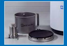
The Cryokit consists of a full metal knife with 4 blades, a stainless steel container with baffles and a special lid.
