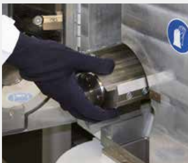
Push fit rotors facilitate quick and easy cleaning
