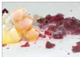
Material embrittled with liquid nitrogen
