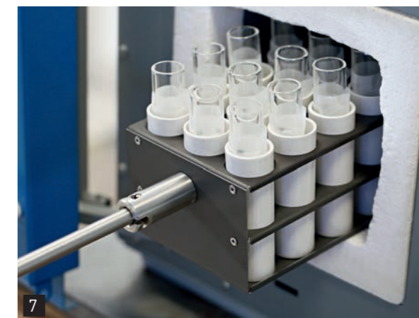
The incinerating module with a long handle makes handling of samples easier.
